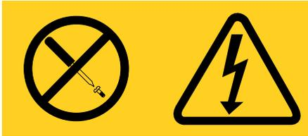
Two warning symbols on a yellow background. The first is a black circle with a diagonal slash over a screwdriver icon, indicating 'no tools' or 'no opening'. The second is a black triangle with a lightning bolt icon, indicating 'hazardous voltage'.
